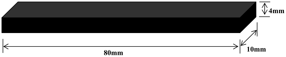
Figure 4. Dimensions of bending specimen (ASTM D 790).
